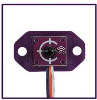
The IR transmitter bit is an output bit that sends data via an infrared (IR) light signal. The IR receiver bit is required to receive the data.
