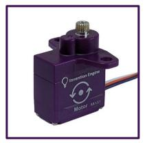
The motor bit is an output bit that rotates an output shaft continuously. For precise angular movements refer to the servo bit.
