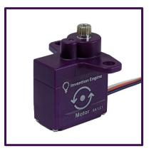
The motor bit is an output bit that rotates an output shaft continuously.
