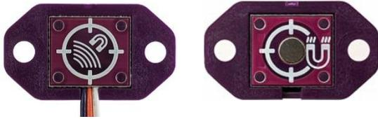
The magnet sensor bit is an input bit that detects the close presence of a magnet. The magnet bit holds a small magnet that can be detected by the magnet sensor bit.
