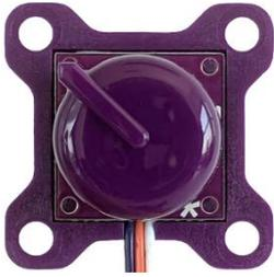
The dial bit is an input bit that allows a user to set a level or number manually.
